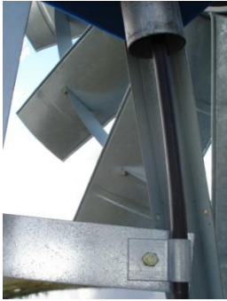
PHOTO 6 – ELONGATED HOSE BRACKET [EHB] AND HOSE BRACKET [HBK] WITH AIRLINE INSTALLED
