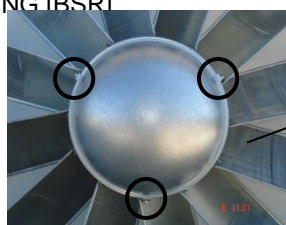
PHOTO 4 - DOME CLIPS (CIRCLED) IN THE CORRECT LOCATION
