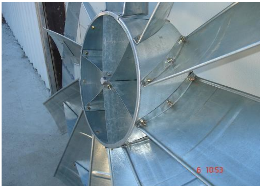
PHOTO 1 - SHOWS THE COMPLETED ASSEMBLY OF THE BLADES [BLD] (FRONT VIEW).
